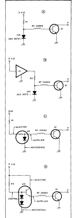
fig. 4. Typical linear biasing schemes. (A) single diode; (B) single diode with 3-terminal regulator U1 (see text); (C) Byistor, BY-1 (see text); (D) Z0-28 (see text). R1 and R2 are power resistors. Q1 is the power amplifier. Q2 is a BY-1 byistor and Q3 is a Z0-28. See text for other component value selections. Note 1: The biasing device must be thermally attached to the power device being controlled.
